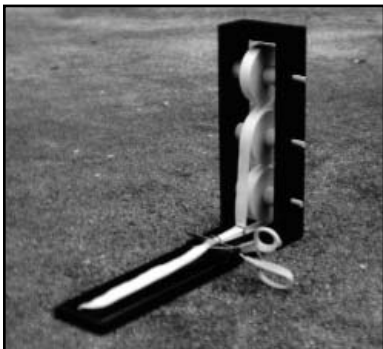
Figure 11. A jig used for dispensing three layers of linen tape to be cut at a time.
