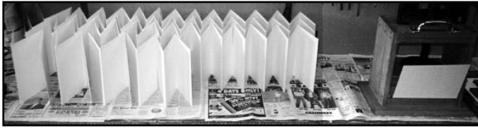
Figure 19. Several double pages drying while another is in the press on the right.
