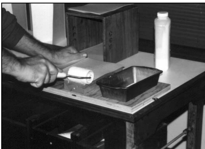
Figure 15. Applying glue to the outer 5/8 of each page with a trim paint roller.
