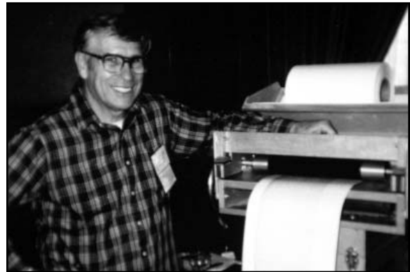
Figure 21. Jack Hewes posing with the book-copying, stencil machine he designed. Note the dark roller on top of the out-coming paper—this is carbon paper turned so that the smudgy portion is on the outside and, therefore, making an imprint on the paper. Photo: Dan Slack archives.
